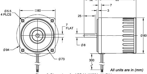
Figure 6: Dimensions for ACP-M-4IK25A-(A)(C)V
