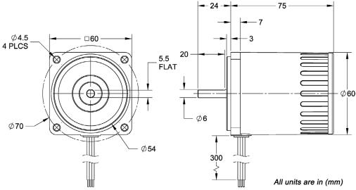
Figure 4: Dimensions for ACP-M-2IK6A-(A)(C)V
