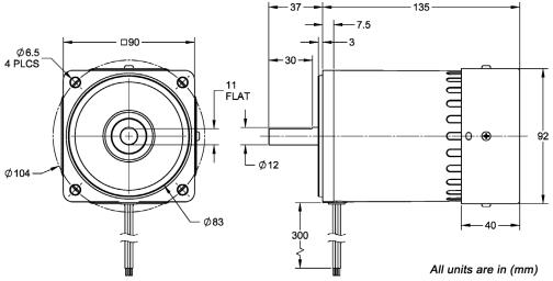
Figure 9: Dimensions for ACP-M-5IK90A-(A)(C)V, ACP-M-5IK120A-(A)(C)V, ACP-M-5IK150A-(A)(C)V
