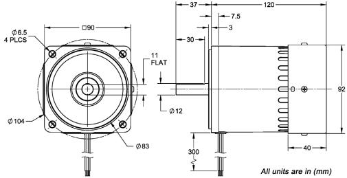
Figure 8: Dimensions for ACP-M-5IK60A-(A)(C)V
