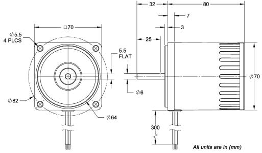
Figure 5: Dimensions for ACP-M-3IK15A-(A)(C)V
