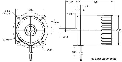
Figure 7: Dimensions for ACP-M-5IK40A-(A)(C)V
